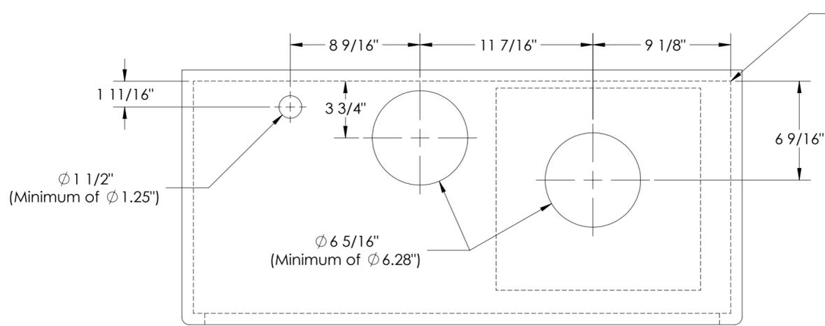
Orientation of all cutouts originate from inside right wall of cabinet. Insert Jet Pack is mounted flush with the right wall and back wall of cabinet.
